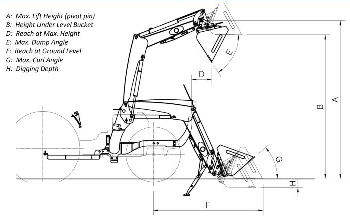
Information listed in this document is the manufacturer's calculated estimates. Values can vary based on machine options, equipment and configuration.
