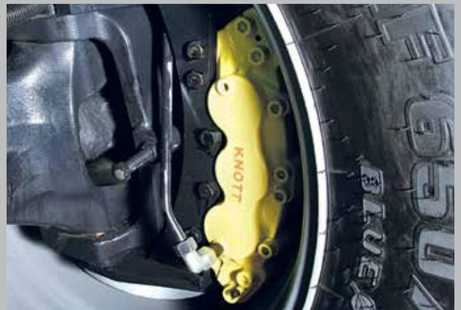
Dry disc brakes on the front axles for extra-safe braking effect (optional).
