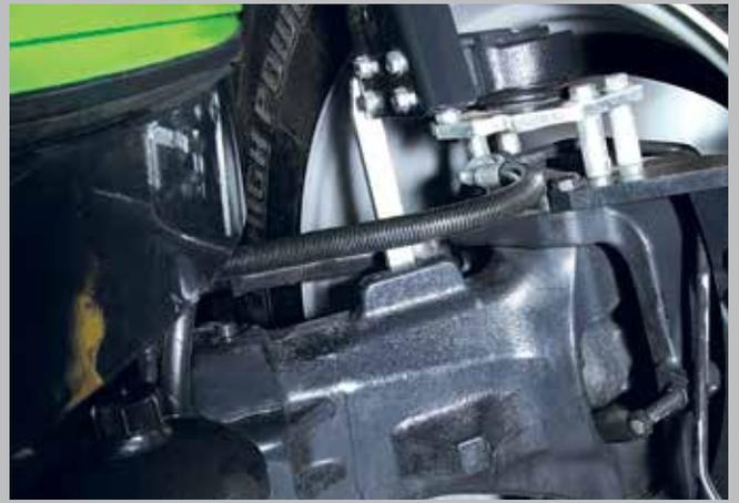
Front axle. Maximum spring effect and a steering angle of up to 50 degrees.
