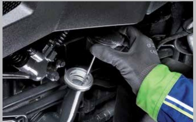
Checking the oil level and topping it up is also incredibly simple.
