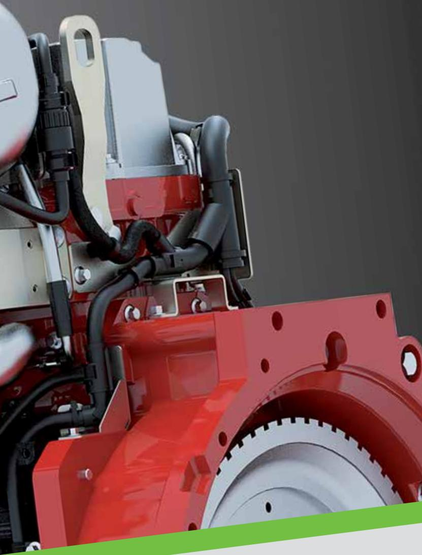
When it comes to the power unit for the 9 Series, only the best is good enough. The decisive factor is the highest performance with the lowest fuel consumption. There is no alternative to the Deutz TTCD 7.8 liter 6-cylinder engine (336 HP) with two-stage turbocharger-, and intercooling as well as SCR, DPF and DCR technology
