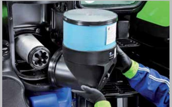
No tools are required for replacing the engine air filter.
