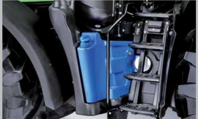
159 gal diesel and 14 gal DEF are sufficient for more than one day of hard work in the field.
