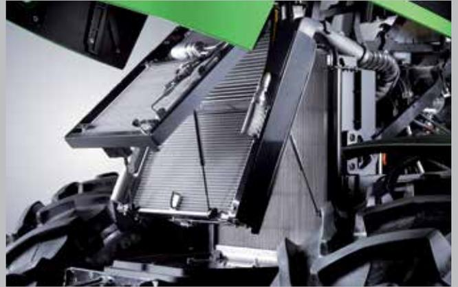
The radiator can be quickly unfolded and cleaned.
