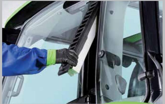
The cab air filter in the cab post can be easily accessed without tools.
