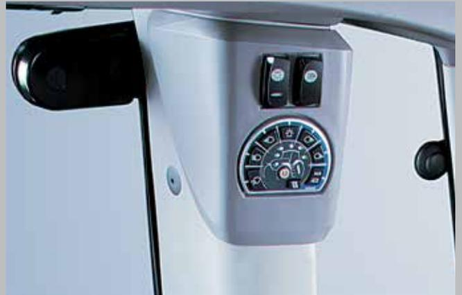
Driving lights, work lights and cab light combined in a single control panel.
