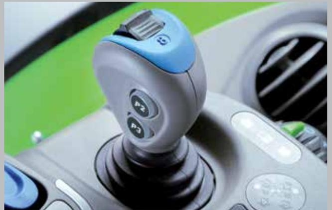
Three hydraulic valves can be controlled via a simple joystick with integrated smart wheel.
