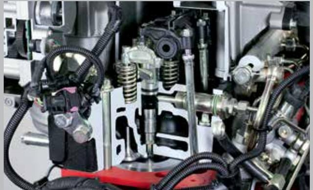
DCR technology. 29,000 PSI injection pressure ensures maximum engine efficiency.
