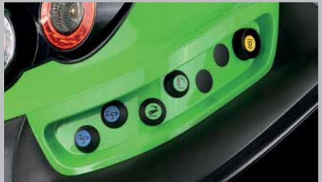
External control for auxiliary hydraulics, rear lift and PTO mounted on both sides of the tractor.
