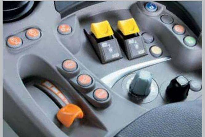
PTO controls (front/rear) are conveniently integrated in the armrest...
