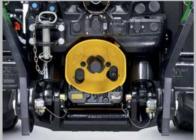
Up to 5 proportional spool valves at the rear and 2 in the front. Front lift integrated to the tractor and closer coupled
