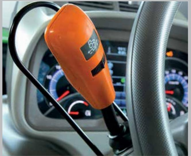
PowerShuttle with SenseClutch - 5 levels of reversing sensitivity that can be easily adjusted.
