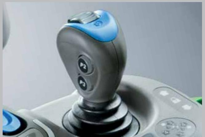
Auxiliary valves are controlled via a joystick with an integrated smart wheel.
