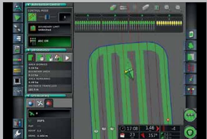
Section control/ variable rate control as standard.
