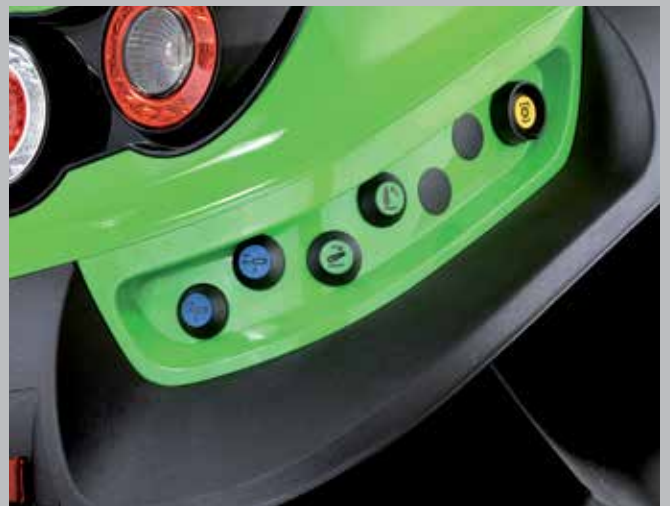
External hydraulic, rear lift and PTO remote controls from each side.
