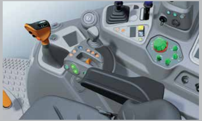
Powershift: The efficient all-round transmission with manual gear changing.
