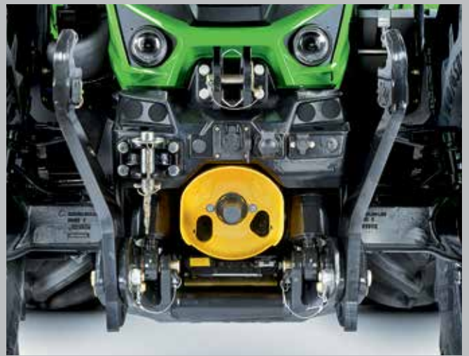
New front lift position control for more work capacity (only TTV models).
