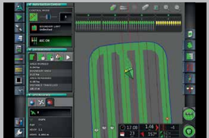
Section control/ variable rate control as standard.
