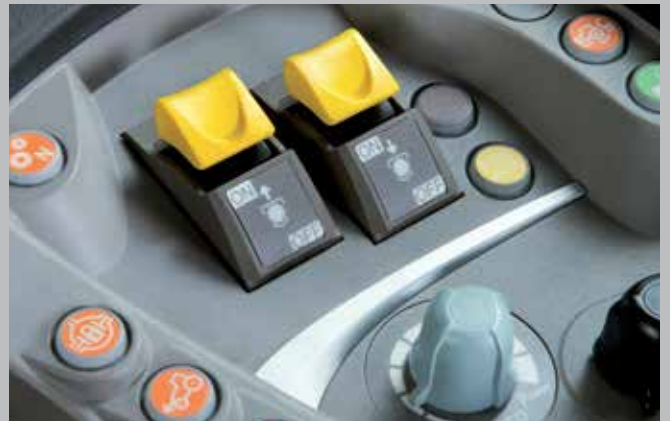
Standard in all cab configurations, the PTO engagement comes with the easy but safe push-button controls.
