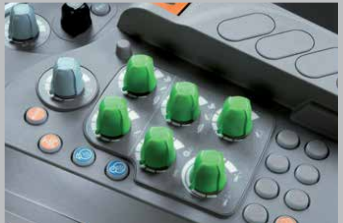
Fine tuning front (TTV only) and rear lift control can be operated through dedicated controls.
