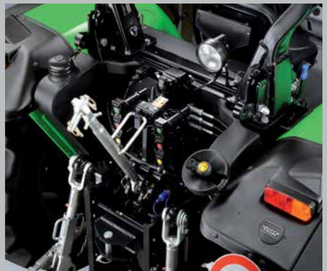
The 14.5 gpm (55 lpm) hydraulic pump supplies up to three rear remote valves.
