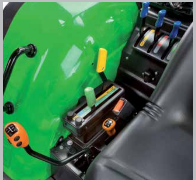
A mechanical transmission with 5 synchronized gears makes for easy shifting on-the-fly to achieve the desired speed.
