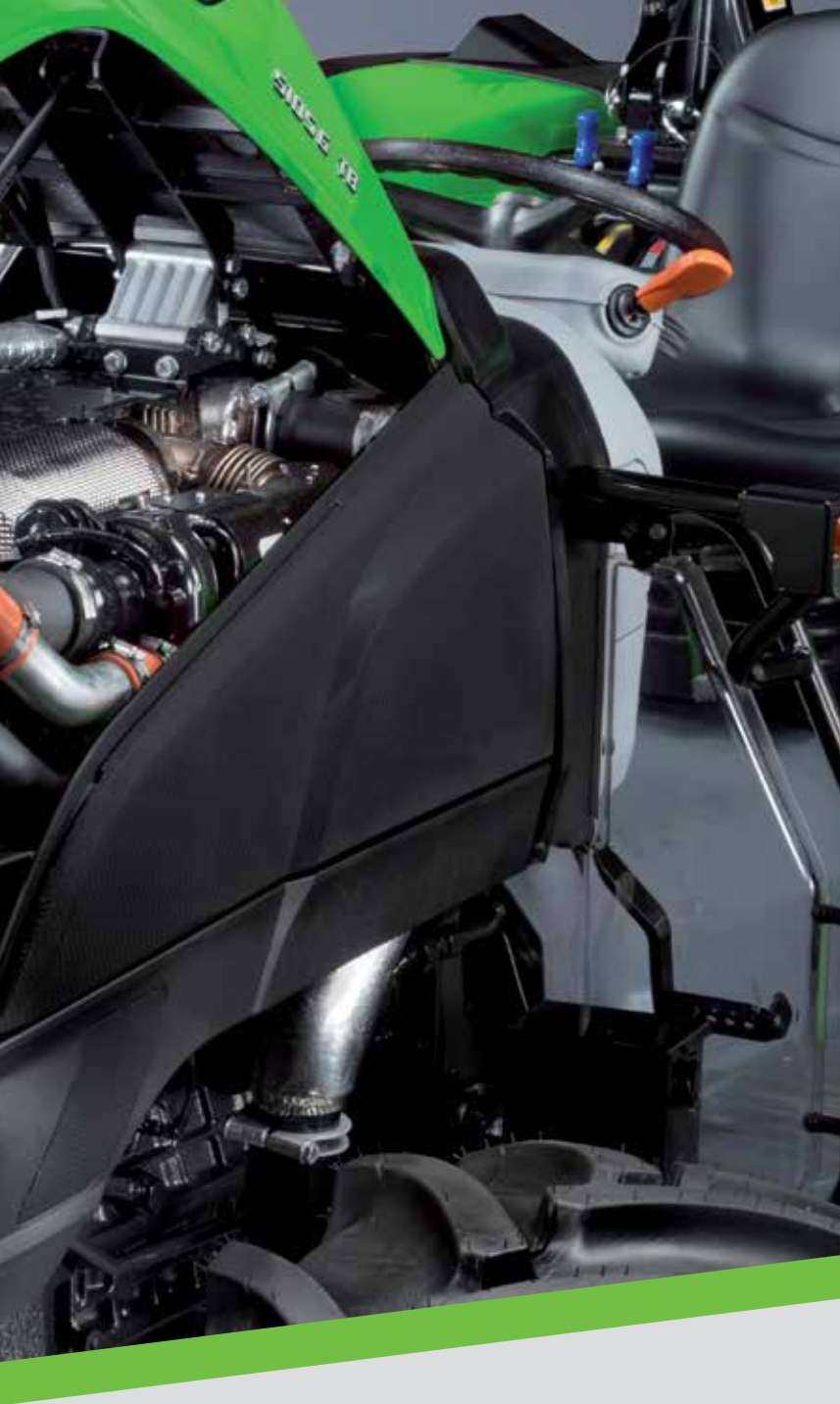
FARMotion engines: constant power and constant torque at low engine speeds without the added emissions complexity of SCR or DPF.
