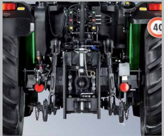
The rear 3-point hitch: up to 7,900 lb (4,525 kg) lifting capacity, extremely precise control. 540/540E rear PTO as standard.
