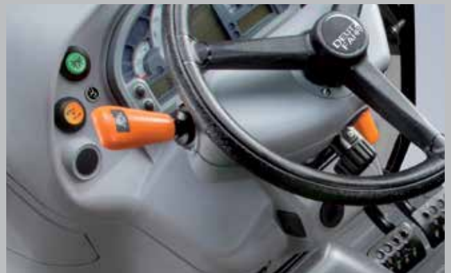
Electro-hydraulic power shuttle with wet multidisc clutch allows the driver to change direction without using the foot clutch pedal.
