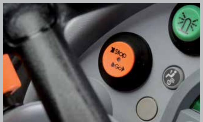
Stop&Go system: stop and start the tractor using only the brake pedal.
