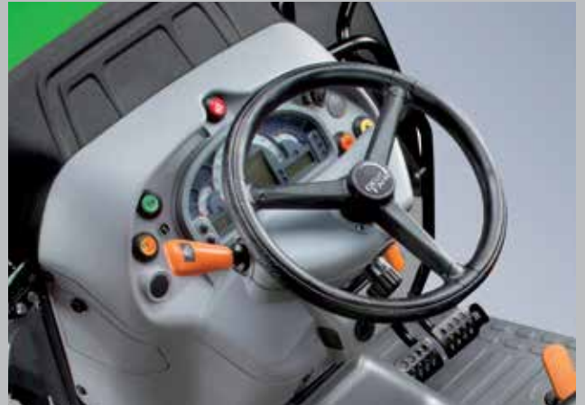
The innovative SSD rapid steering system halves the number of steering wheel turns to the full steering angle.
