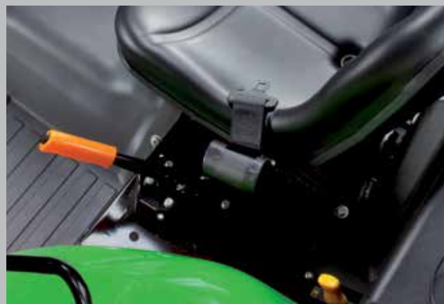
To the left of the driver: parking brake and PTO controls.
