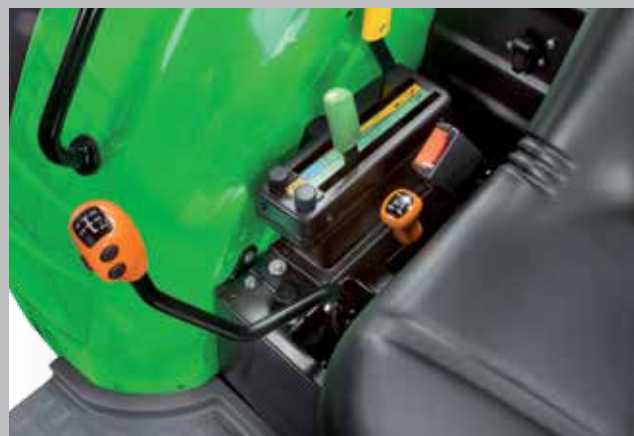
To the right of the driver: gear lever, rear power lift and hydraulic control units ergonomically organized.
