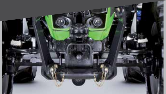
Front lift and PTO. Lifting capacity of 4,625 lb and 1,000 PTO.
