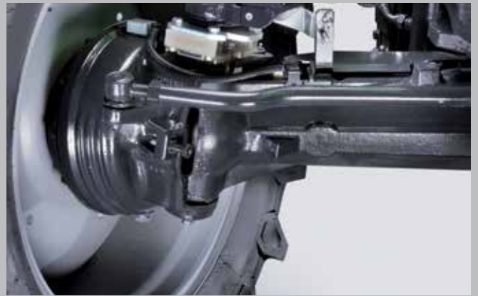
A unique safety concept from DEUTZ-FAHR. Separate oil cooled disc brakes in the front axle.
