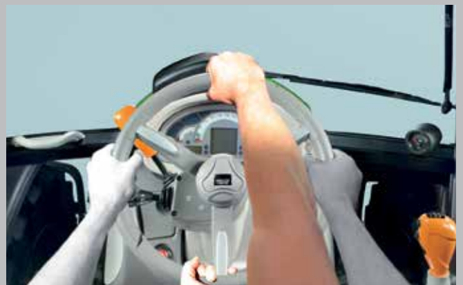
The SDD fast steering system. Half the steering wheel rotations, double the steering speed.
