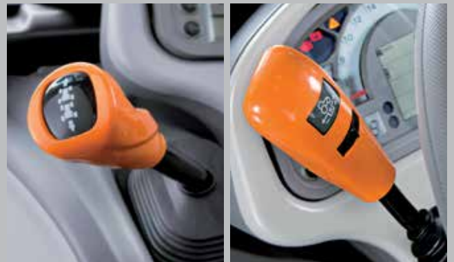
Mechanical reverse shuttle or power shuttle with five adjustable settings – the choice is yours.
