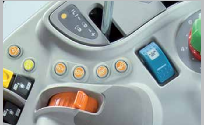
Push button operation of the 4wd and diff. lock engagement: maximum comfort and maximum performance.
