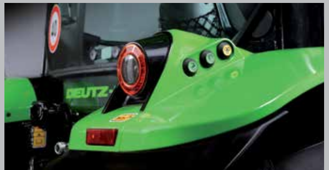
External PTO and hitch controls for straight forward equipment mounting and external equipment operation.
