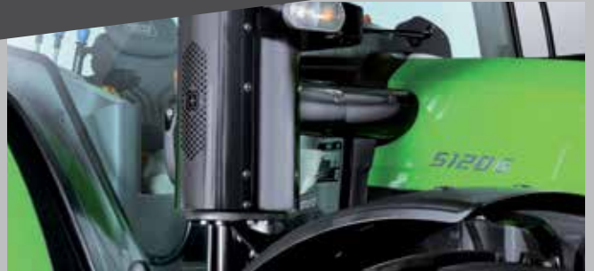
State-of-the-art selective catalyst reduction (SCR) exhaust technology is simple and reliable.
