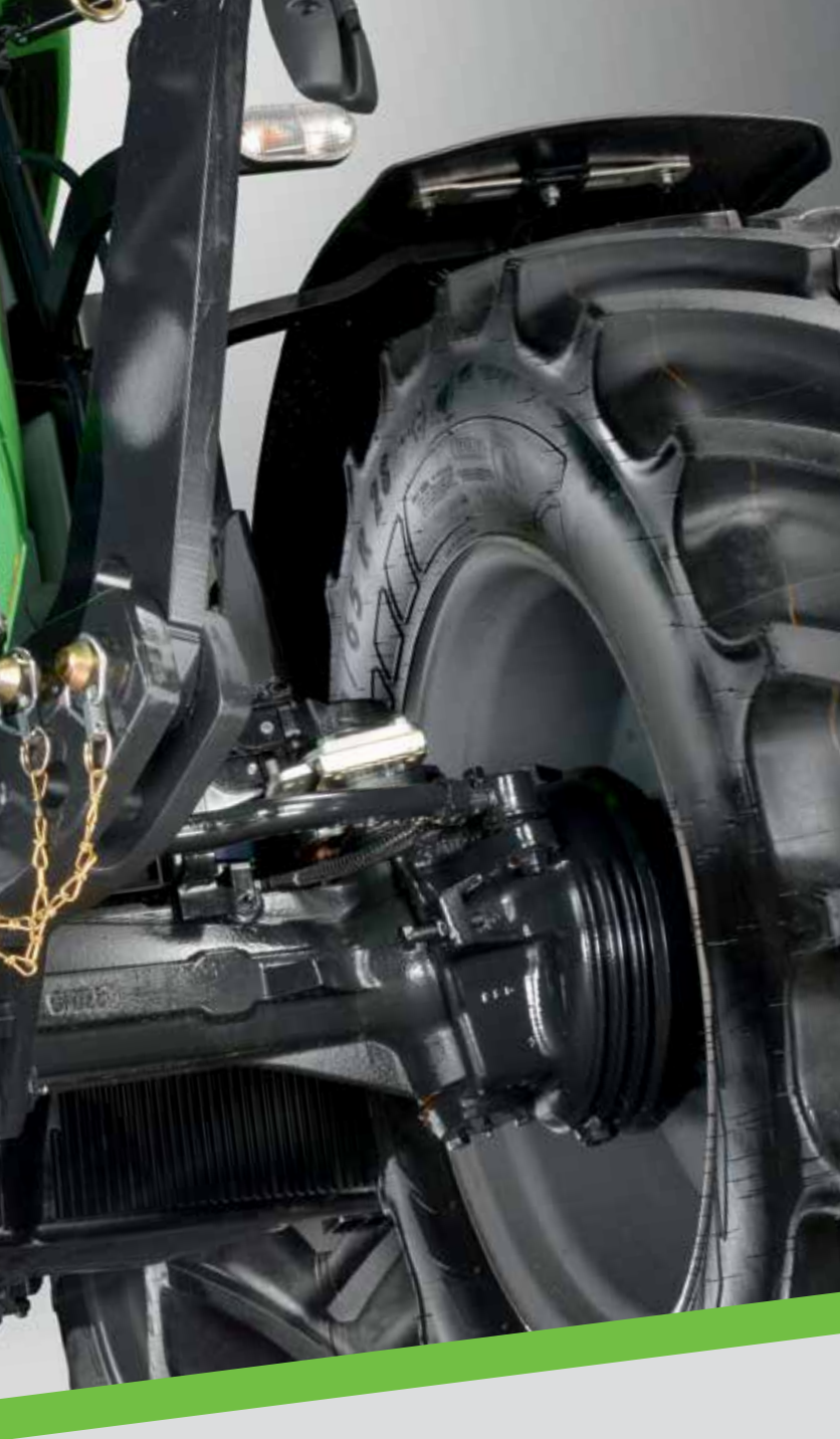
A unique safety concept from DEUTZ-FAHR. Separate oil cooled disc brakes in the front axle.
