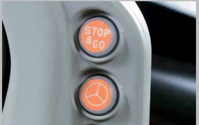
Convenient Stop&Go, as well as steering double displacement (SDD) rapid steering system ...
