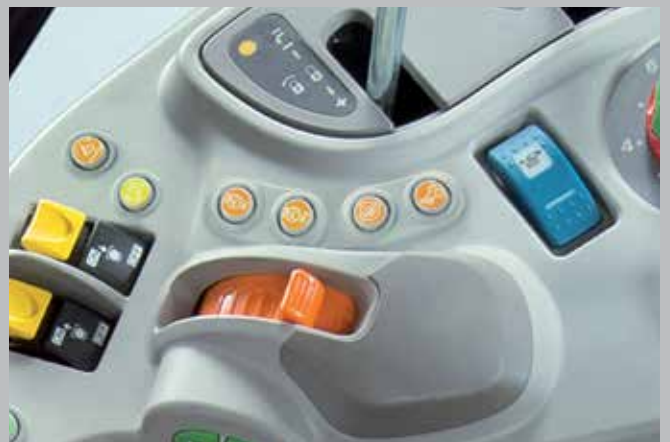
New: two engine speed settings. Pre-programmed efficiency for routine operations.
