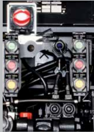
Up to 3 hydraulic remote valves at the rear and 2 sets of couplers near the front.
