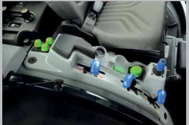
Hydraulics and rear power lift controls. Neatly arranged to the right of the seat.
