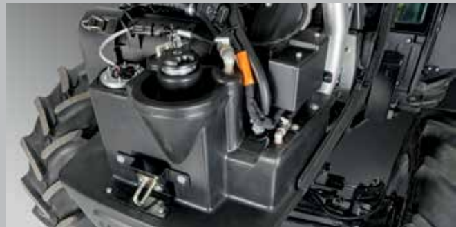
The fuel tank built into the front axle block can be filled with the bonnet closed, while an additional tank is located below the chassis.
