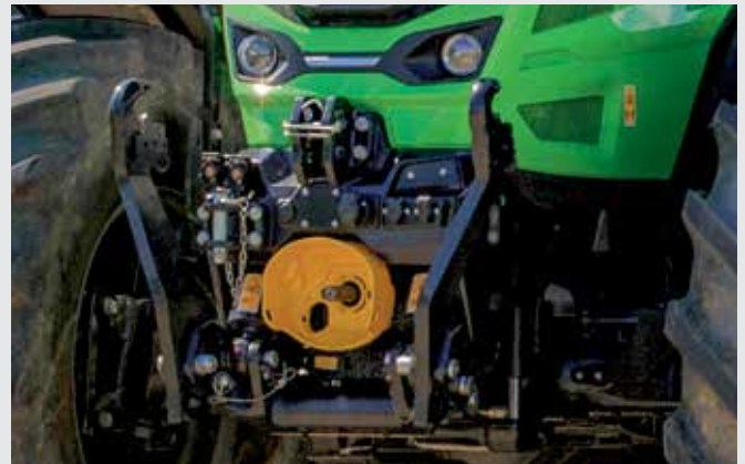
5,450 kg lifting capacity and dual speed front PTO.
