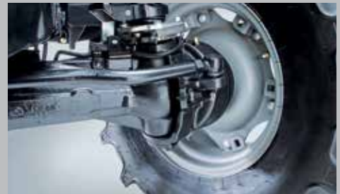
Electronically activated four-wheel drive and 100% differential lock, four-wheel brake and 55-degree steering angle.
