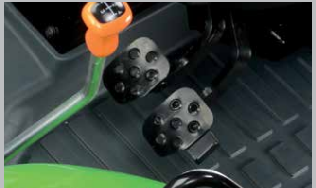
4-wheel braking with wet disc brakes.
