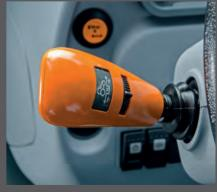
**Standard:** Hydraulic power shuttle system. The shuttle sensitivity (hard – medium – soft) can be easily adjusted with the thumb.
