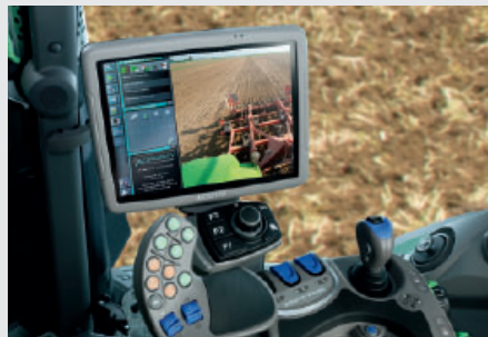
Integrated camera with automatic full screen mode (e.g. reversing) for a clear overview and safety.
