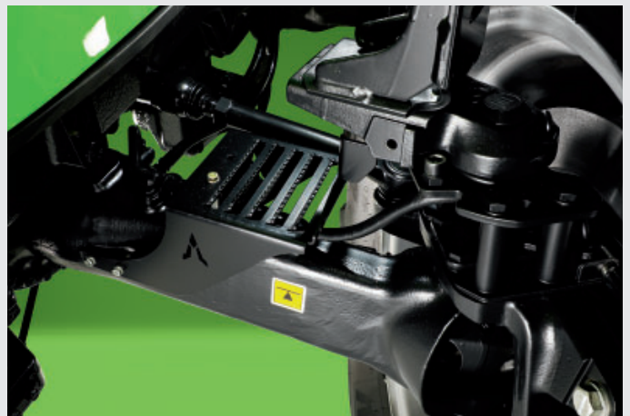
↑ Maintenance steps above the front axle for comfortable cleaning.
