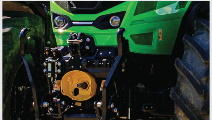
↑ 12,015 lb lifting capacity and dual speed front PTO.
