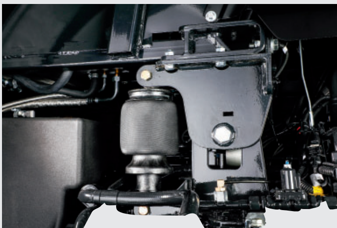
↑ Pneumatic cab suspension for a smoothest ride.
