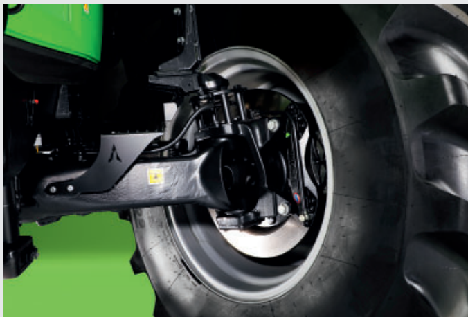
↑ Dry disc brakes for maximum brake performance.
