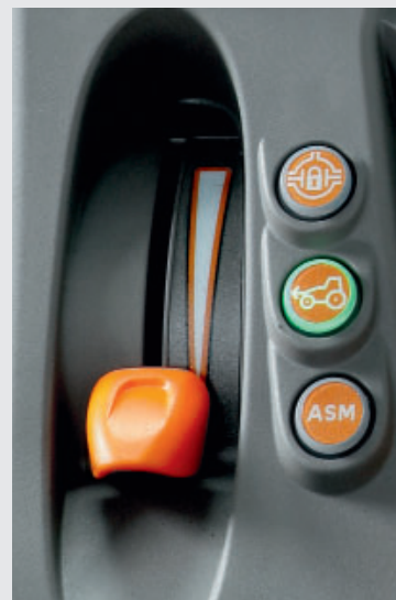
↑ Electro hydraulically operated 4WD and differential lock including ASM
