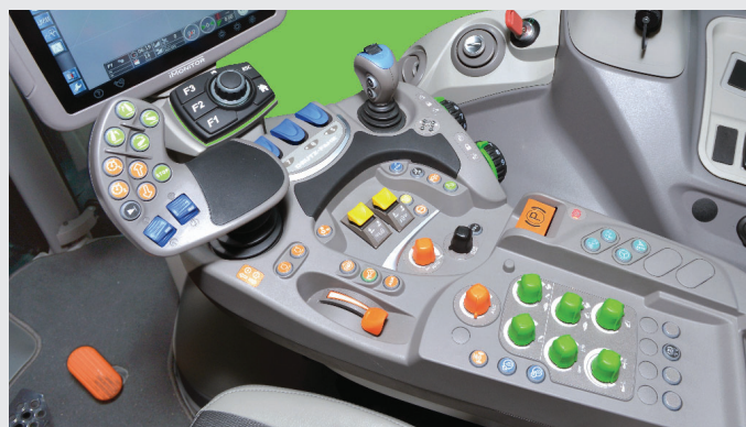
Proven DEUTZ-FAHR layout. Functions grouped into colours for intuitive operation.
