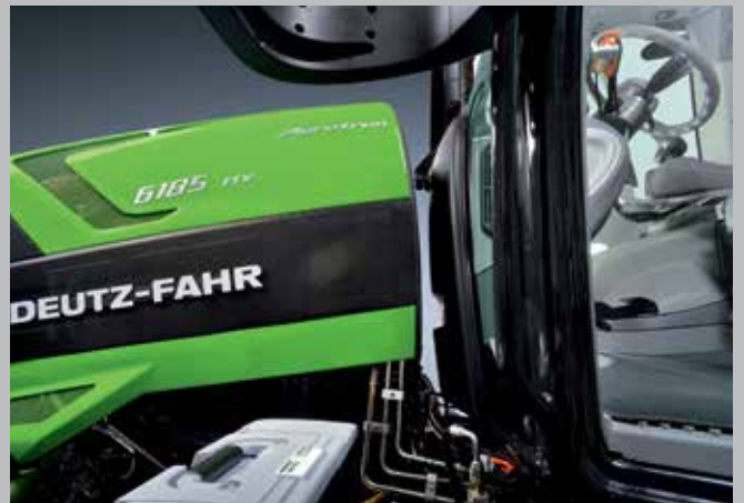
No connection between cab and engine hood - improved driver comfort.
