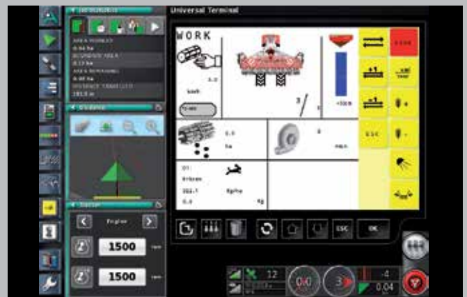
TIM ready (Tractors Implement Management) functions can follow implement functionality.
