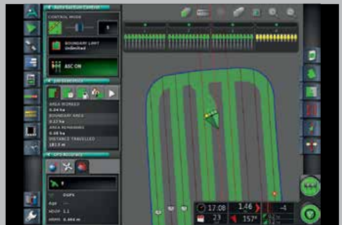
Section control/ variable rate control as standard.
