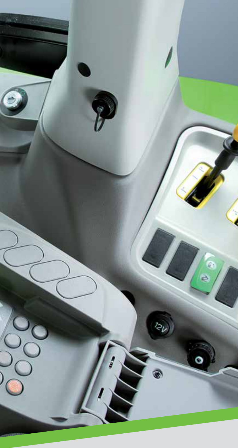
Hydraulic valves can be managed through proportional and programmable controls. The electronic Joystick can be programmed to use the front-loader and other tractor functions with the thumbwheel.
