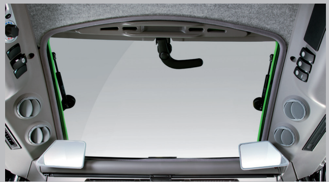
A transparent opening sunroof provides unobstructed view of a fully raised loader.
