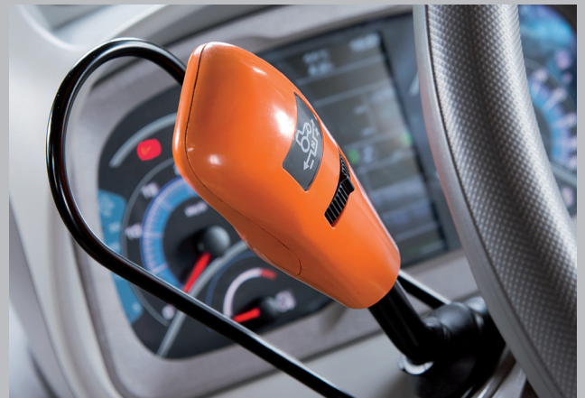
Powershuttle with 5 adjustable settings for changes of direction without interruption of torque.
