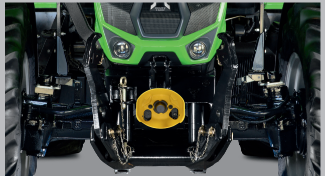
The powerful front linkage can lift up to 6,300 lb: optional equipment.
