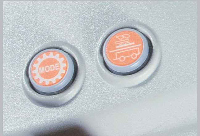
Two working modes (FIELD/TRANSPORT) can be selected with push button.
