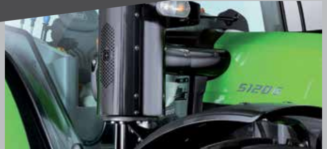
State-of-the-art selective catalyst reduction (SCR) exhaust technology.
