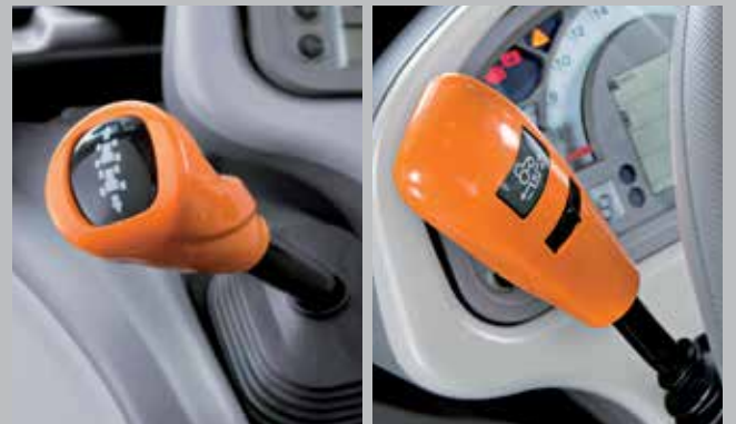
Mechanical reverse shuttle or Powershift with five adjustable settings – the choice is yours.
