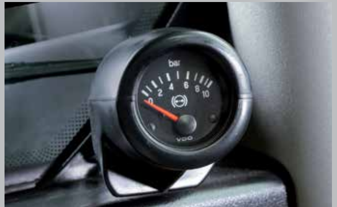
Air brake system (optional) for reliable braking of heavy rear towed equipment.
