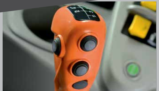
Comfort clutch and Powershift. Simply change gear at the push of a button without pressing the clutch.
