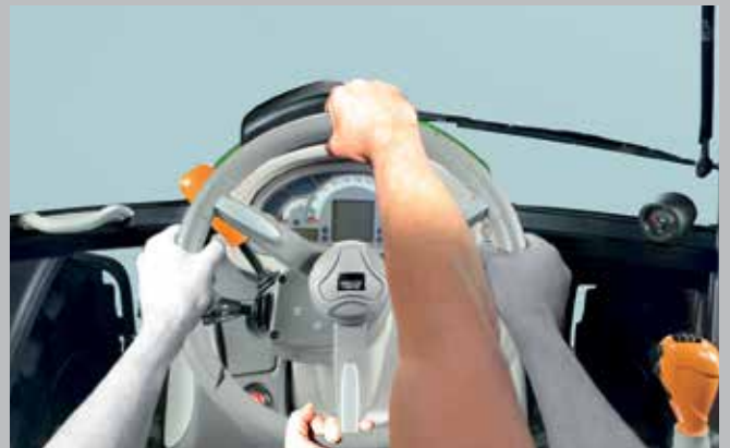
The SDD rapid steering system. Half the steering wheel rotation, double the steering speed.
