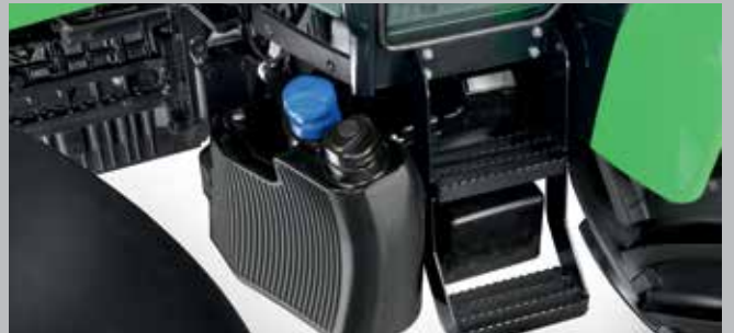
A fuel tank that holds up to 38.3 gallons and 2.5 gallons of DEF, allows long working periods. (depending on model)
