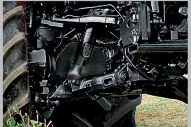
Independent wheel suspension with double wishbone design.
