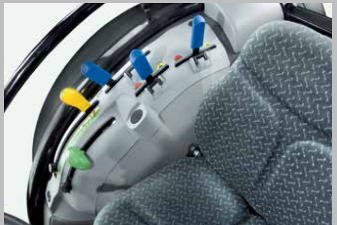
Mechanical rear lift levers, functional and ergonomic.
