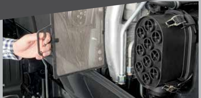
Engine efficiency is aided by the large, newly designed cooling package, improved air flow and the Powercore air filter.
