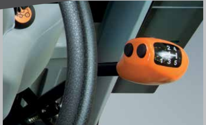
Power shift. Change gears at the push of a button without depressing the clutch.
