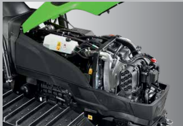
FARMotion diesel engine delivers high torque with "No Maintenance" emissions.
