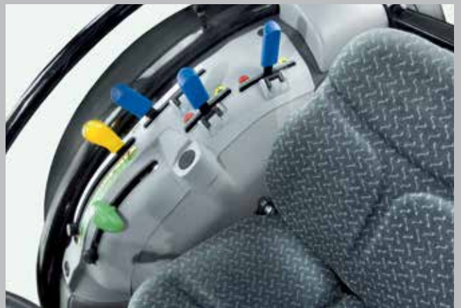
Mechanical rear lift levers, functional and ergonomic.
